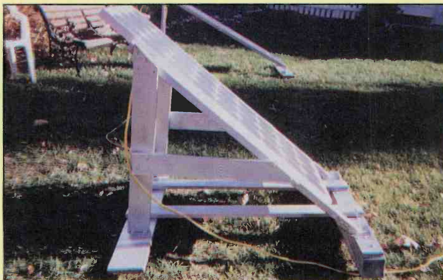
A side view of the large Siemens panel mounted on the homebrewed wooden frame.
