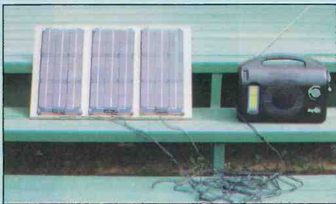
The SolarVerter panels, wired in parallel, mounted on a piece of 24" x 15" wood and connected to the BayGen Freeplay radio.
