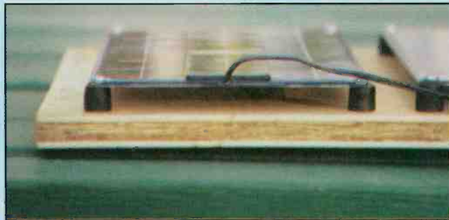
A side view of one of the SolarVerter panels showing the mounting grommets obtained at a local hamfest. The small, efficient panels are waterproof and can be mounted outdoors.
