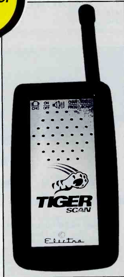
The Tiger Scan represents a very interesting, but simple scanner. Easily portable and quick to reprogram, it makes for a versatile monitor in the VHF High band.
