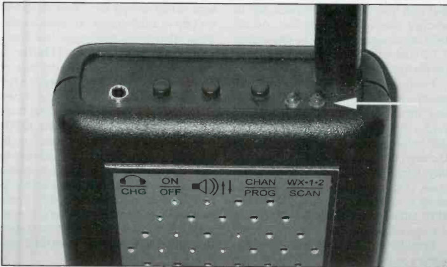
There are very few controls on the Tiger Scan. On/Off, volume, and Channel select/Program are the three buttons. The arrow points to the channel indicator lights — both of them.
